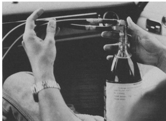
Fuel from special containers is fed to engine of Hugh Whitted's diesel automobile during a fuel mileage test. Average result on three tests on each type of fuel showed 37.62 miles per gallon on No. 2 diesel fuel and 35.86 miles a gallon on crude peanut oil. (Photographs courtesy of Hugh Whitted).
