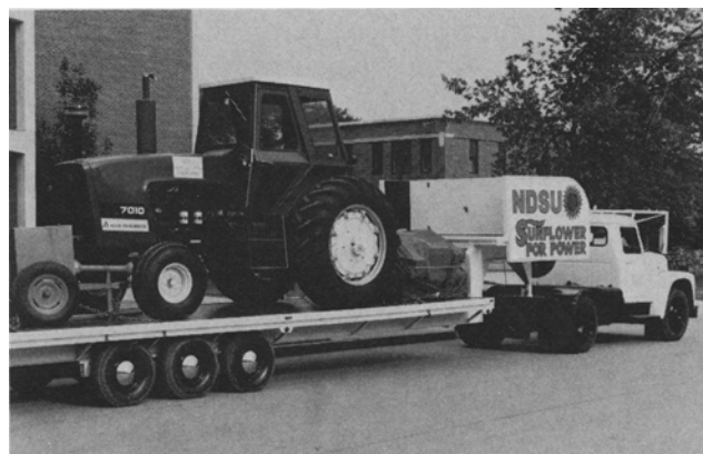
North Dakota State University's mobile demonstration unit, "Sunflower for Power," has toured most of that state demonstrating that a modern tractor can be operated on pure sunflower oil.
