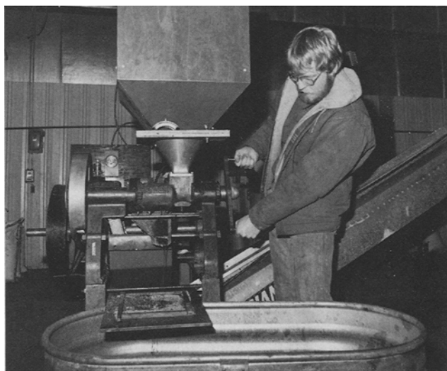
Vance Haugen, a research technician at North Dakota State University, adjusts screw press as oil is extracted from sunflower seed. (North Dakota State University photographs courtesy of Harold Caldwell, NDSU extension service).
